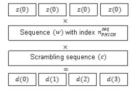
The variable w is an orthogonal scrambling sequence with index  $n_{P\!H\!ICH}^{seq}$ . The sequences are given in the following table.
