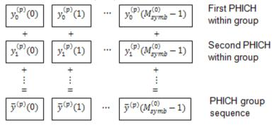
The variable  $y_i^{(p)}(n)$  is the *n*-th element within PHICH *i* on antenna port *p*.
