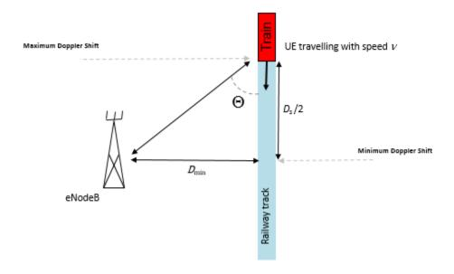
The expression  $D_s$  /2 is the initial distance of the train from eNodeB, and  $D_{\min}$  is the minimum distance between eNodeB and the railway track. Both variables are measured in meters. The variable v is the velocity of the train in meters per second. The Doppler shift due to a moving train is given in the following equation.
