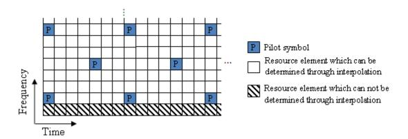
In this case, channel estimates at the edges cannot be interpolated from the pilot symbols. To overcome this problem, virtual pilot symbols are created. The function lteDLChannelEstimate creates virtual pilot symbols on all the edges of the received grid to allow cubic interpolation.
