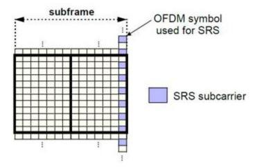
The minimum frequency span covered by the SRS in terms of bandwidth is 4 resource blocks and larger spans are covered in multiples of 4 resource blocks. This means that the minimum sequence length is 24. To maximize the number of available Zadoff-Chu sequences, a prime length sequence is needed. The minimum length sequence, 24, is not prime.
