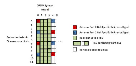
Cell-specific reference signals are present within the first OFDM symbol. As four REs not containing cell specific reference signals are required in a REG, the twelve REs in the first symbol are divided into two REGs, each containing six REs (two containing cell specific reference signals and four empty). In the second and third OFDM symbols no cell specific reference signal is present therefore the twelve REs in each symbol are divided bewteen three REGs, each containing four REs.
