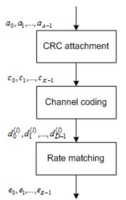
To form the PDCCH payload, the DCI undergoes coding as shown in the following figure.
