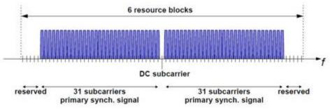
As the DC subcarrier contains no information in LTE this corresponds to mapping onto the middle 62 subcarriers within an OFDM symbol in a resource grid. d(n) is mapped from lowest subcarrier to highest subcarrier. The PSS is mapped to different OFDM symbols depending on which frame type is used. Frame type 1 is frequency division duplex (FDD), and frame type 2 is time division duplex (TDD).
