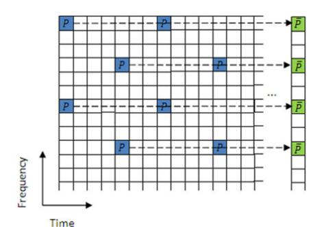
All the pilot symbols found in a subcarrier are time averaged across all OFDM symbols, resulting in a column vector containing the average for each reference signal subcarrier,  $\bar{P}$
