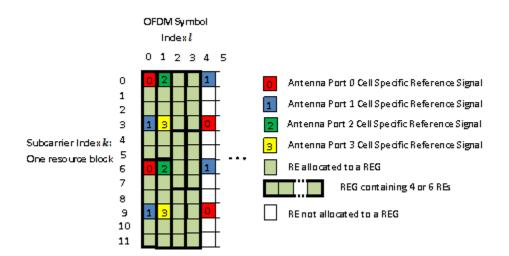
The REG allocation within the first OFDM symbol is the same as for a one or two antenna port configuration. Four cell specific reference signals are present in the second OFDM symbol therefore eight REs are available for the mapping of control data. The twelve REs are divided into two REGs, each containing six REs. The third and fourth OFDM symbols contain no reference signals so three REGs are available.
