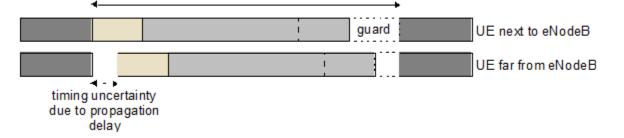
Therefore the size of the guard period determines the cell radius, as any propagation delay exceeding the guard time would cause the random access preamble to overlap the following subframe at the eNodeB receiver.
