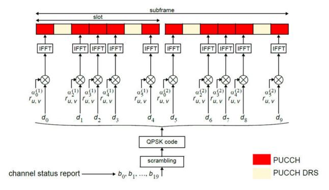
The cyclic shifted sequence applied to randomize intercell interference is denoted here by  $r_{u,v}$ . For extended cyclic prefix, where there are only six SC-FDMA symbols per slot, the mapping to resources changes slightly. In this case, only one reference signal is transmitted per slot, and the signal occupies the third symbol in each slot.
