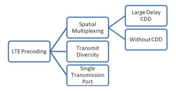
The precoder takes a block from the layer mapper,  $x^{(0)}(i), x^{(1)}(i), \dots, x^{(v-1)}(i)$ , and generates a sequence for each antenna port,  $y^{(p)}(i)$ . The variable p is the transmit antenna port number, and can assume values of  $\{0\}, \{0,1\},$  or  $\{0,1,2,3\}$ .
