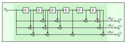
Each output stream of the coder is obtained by convolving the input with the impulse response of the encoder, as shown in the following equation.
