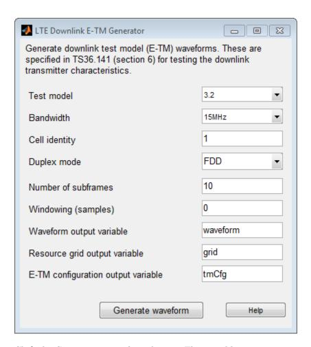
Click the  $Generate\ waveform\ button.$  The variables waveform, grid, and tmCfg now appear in the MATLAB Workspace Browser.
