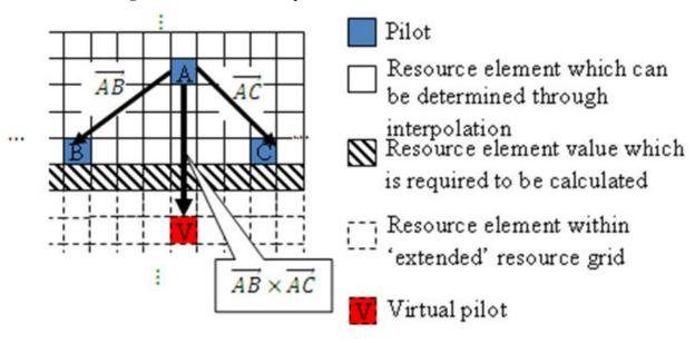
Note  $\overline{\text{Virtual pilots}}$  are only created for the MATLAB® 'linear' and 'cubic' interpolation methods.
