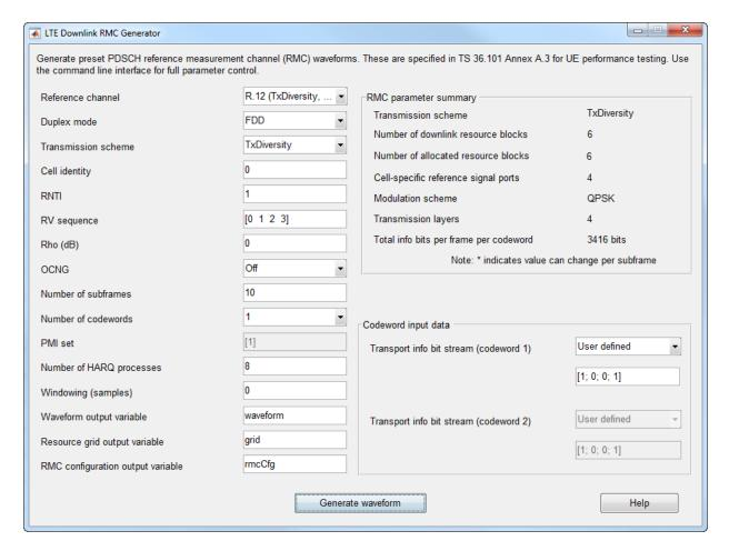
Click the **Generate waveform** button. The variables waveform, grid, and rmcCfg now appear in the MATLAB Workspace Browser.
