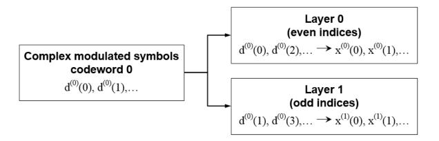
• **Two Codewords** — Codeword 0 is mapped to layer 0 and codeword 1 is mapped to layer 1, as shown in the following figure.
