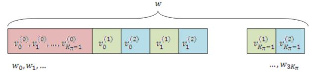
Interlacing allows equal levels of protection for each parity sequence.
