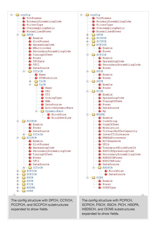
**Note** Each instance of the CCTrCH substructure contains the same fields, so the contents is only expanded in the first appearance the figure.
