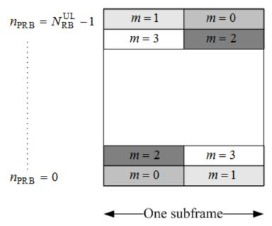
The resource for PUCCH formats 2, 2a, and 2b is indicated by a single scalar value called resource index. From this value, the cyclic shift can be determined. Time and frequency allocated resources are not derived from this value. However, higher layers are in full control of when and where control information is transmitted.
